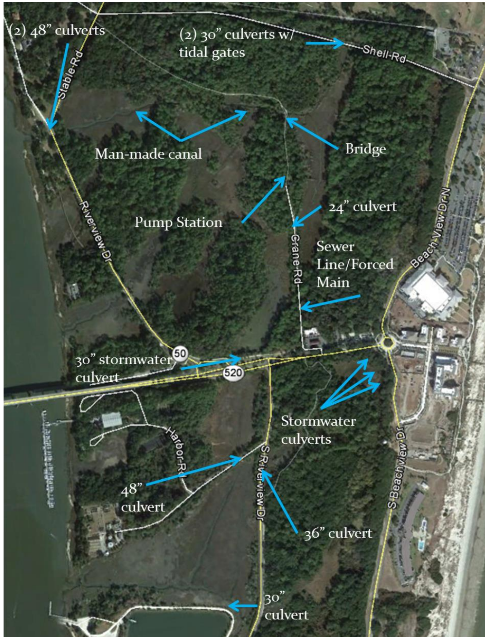
Figure 2. The current First Creek system with specific locations of altered connectivity including road/bridge obstructions, culvert systems and channel alterations.
